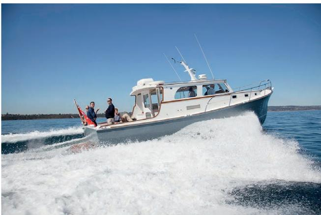
Powering her is a single Yanmar 530Hp Diesel, which drives a swept back, five-bladed screw with variable pitch inserts. 2000 litres of fuel and a 1 metric tonne of water ensure you'll be able to look at some serious blue water cruising or have a few very luxurious days afloat, as you hop up the coast somewhere.
